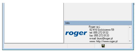
Figure 2.1. The floppy disk icon on the status bar informs about the need to make system backup
